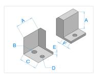
The aluminum bracket is attached at the end of series 30 profiles, where the large M8 hole (drawing B) makes it easy to mount casters / transpor wheels or a foot. Only a single M8 bolt and a T-nut are needed to secure it.
