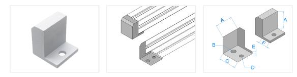
Aluminum end fitting with M6 hole, mounted at the end of a Series 20 profile. Can be used for a foot or transport wheel. Only a M6 bolt and T-nut, or hammer bolt and nut are needed for installation. Buy online at: www.matronics.eu/A200221
