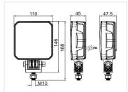
The latest generation of LED lamps constructed in ThermoPlast. Both the housing and the bracket are made of this material. This ensures that the lamp is not affected by weather conditions and maintains a nice surface even when exposed to wind and weather.
