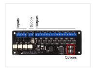
Controller with 8 channels for dynamic indicators and strobe light, as well as positions lights with posibility of dimming.
