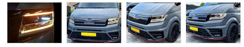
Complete conversion kit for MAN TGE / VW Crafter with LED headlights from 2020+, to replace the cold white LED DRL with yellow/orange light. The 10 bright high power LEDs create an equivalent brightness to the original.
