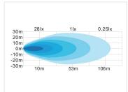
With its oval design and low height, this 10W LED worklamp is an obvious choice to sit on doorsteps on trucks or other places, where space is lacking. The worklamp has 2 powerful 5W CREE LED's, that provide up to 700 raw lumen.
