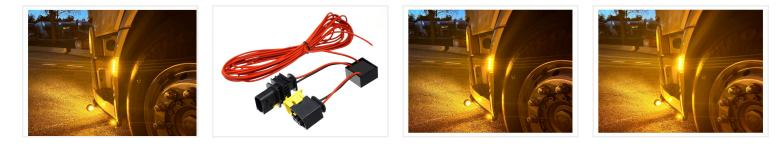
Simple adapter, so that you can use the indicators on the side of the cabin, as a position light. The brightness will be dimmed compared to the indicator light. The indicator will work as usual with its high brightness, and it is still highly visible due to the difference in brightness.
