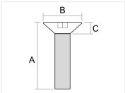
Standard countersunk bolt with M4 thread. Used in brackets, hinges etc. where you need a flush surface
