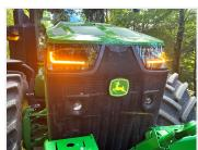
Complete conversion kit for John Deere R series with LED headlights from 2020+ to replace the cold white LED DRL light. The bright high power LEDs give you plenty of light. They are mounted on an aluminum plate like the original, which ensures optimal cooling and extended lifetime on the LEDs.
