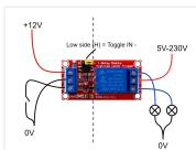
Simple relay module that can be used where you have a low-voltage-signal, that has to turn on or off a higher voltage.
