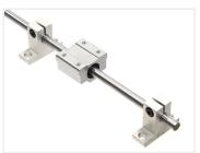
Linear block for 8mm axle, with holes for mounting of part, typically called SC8UU. There are 4 rows of balls inside the block, which gives you an even and precise movement.
