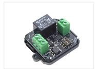
Simple light timer, that is very easy to connect and adjust. The timer Turns on the output, when activated, eg. with a switch. It turns off after set time, or when you push the button again.
