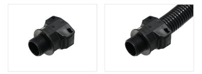
Gland for NW17 tubes, with M20 thread. The tube is pushed in and locks itself. The gland is fastened with a M20 nut.
