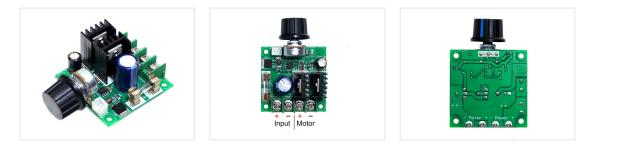
Motor-controller for small and large motors, with max 10A. Easy adjustment of speed with the dial. The dial can easily be mounted in a panel.
