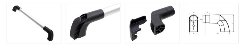
Large handle for series 40 profiles. The anodized Ø30mm aluminum tube can be cut off to the wanted length and is then put into the ends, which are fastened with M8 bolts. The plastic ends are made of reinforced nylon for maximum durability.
