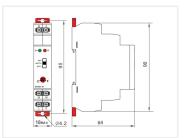
Light-sensor relay for mounting on DIN-rail, that for example can be used for turning on lights during nighttime.
