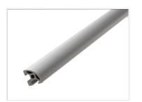
Profile with base measures 20x20, with two of the corners rounded, so that the profile has a quarter-circle shape. There is T-slot on 2 sides, while the 2 other sides are completely flat rounded.
